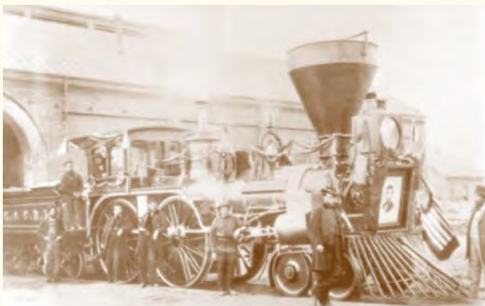
This 4-4-0 steam locomotive drew Lincoln’s Funeral Train. (The “4-4-0” means 4 leading wheels, 4 driving wheels, and 0 trailing wheels.)
